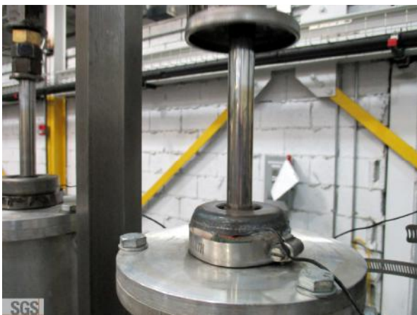
Photograph #7: Birkom#2, rod discoloration at 219,866 cyc.
