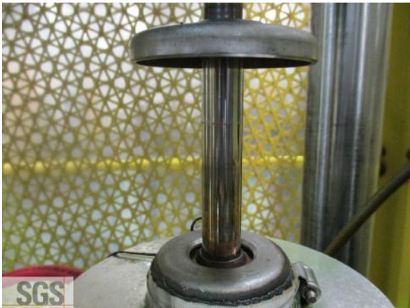
Photograph #5: Birkom#1, rod discoloration at 50,610 cyc.
