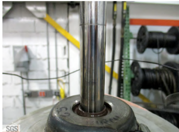
Photograph #6: Birkom#2, rod discoloration at 34,692 cyc.
