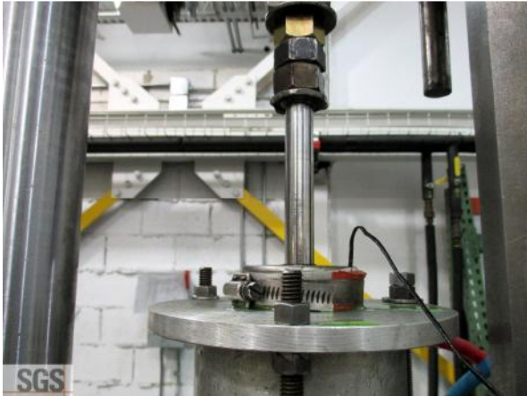
Photograph #3: Comparison Shock Rod discoloration at 82,655 cyc.
